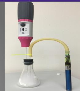
In order to simulate second hand smoke, a "hookah" was set up to draw the vapors onto a piece of cotton soaked in a 2:1 Benzene:Ethanol mixture to extract the compounds for GC-MS analysis
