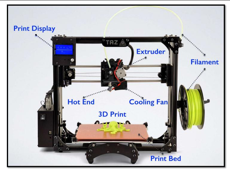
Filament: Material used to build 3D printed parts
