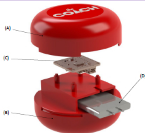
Figure 4. Exploded View of The Coach with the Top Housing (A), Bottom Housing (B), Razor (C), and Battery (D)
