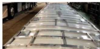
Figure 3. Foretravel ih-45 aluminum frame
