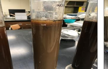
Measuring with a Hydrometer for Soil
