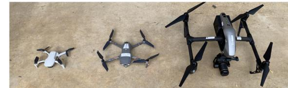
Figure 9. (Left to right) DJI Mini 2, (quiet, but more readily subject to 'blow away'), DJI Mavic 2 Enterprise Advanced (thermal camera  $\pm 2^\circ\text{C}$  temperature measurement accuracy), DJI Inspire 2 (wind resistance, can handle ocean air currents, high resolution camera, dual pilot controls, standard on marine mammal research).
