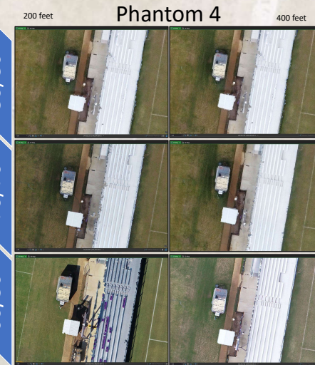
Figure 5 – Orthophotos from a Phantom 4 at various heights and overlaps percentages
