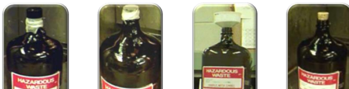
Examples of Improper Container Capping
