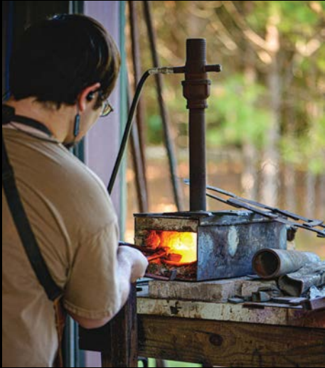
Kevin Burgess heats the steel inside his homemade forge.
