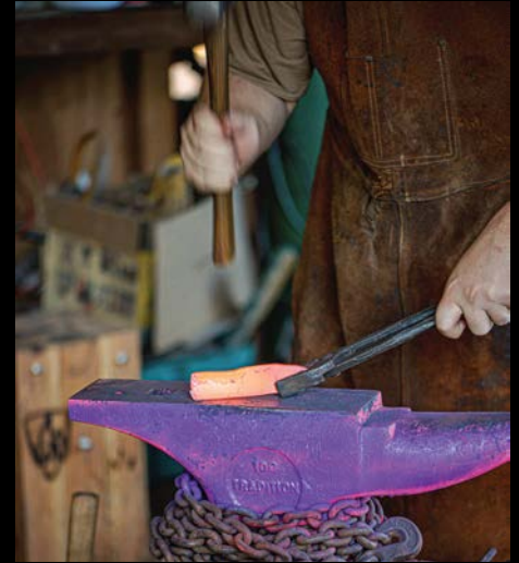
Burgess beats the pliable steel with the help of a steel hammer and a cast iron anvil.
