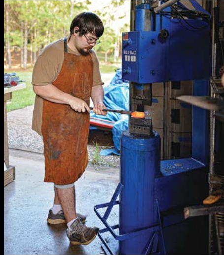
He hammers the hot steel using the Blu Max 110, affectionately known as Big Blue.
