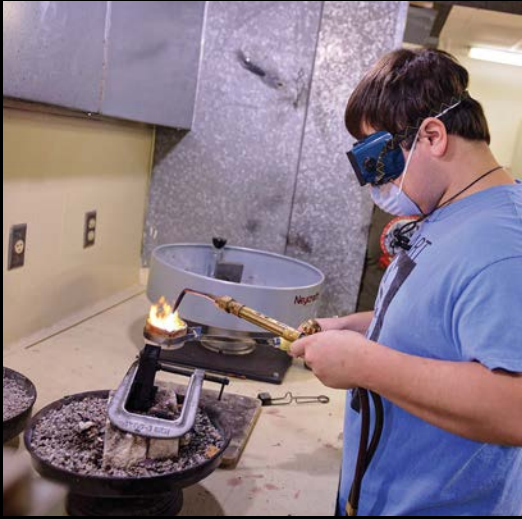
Burgess recycles sterling silver scraps by melting them in a crucible and pouring the metal into a wire ingot mold during his SFA metalsmithing class.
