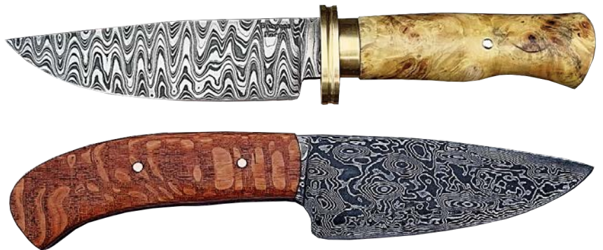
Burgess' specialty is Damascus steel knife blades. Damascus steel is a famed type of steel recognizable by the watery or wavy light and dark pattern of the metal. Aside from being beautiful, Damascus steel is valued because it maintains a keen edge, yet is hard and flexible.
