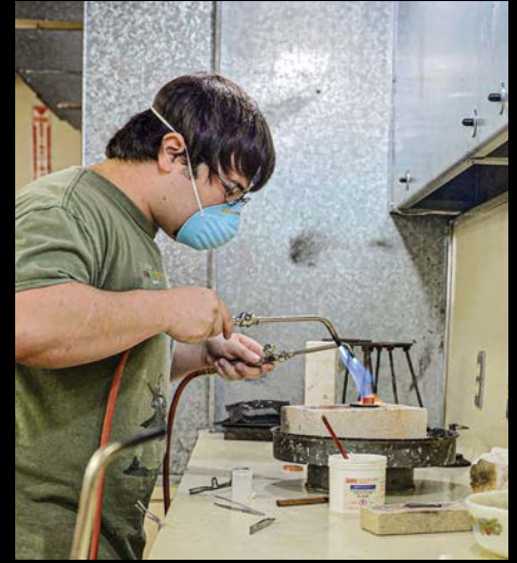
Using two air/acetylene torches, Burgess silver solders a hollow construction ring.
