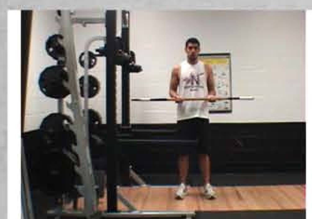
The subject must be recorded holding a scaling rod as part of the videotaping procedure. This allows the software to accurately calculate life-size distances.
